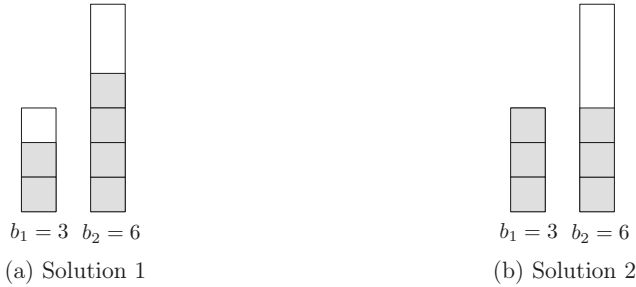
Figure 4.1: Two possible solutions for an instance with two knapsacks and six items, each with weight 1, for \eta = 2/3 . The left solution has an average utilization ratio of 2/3 , exactly equal to \eta . The right solution has an average utilization ratio of 3/4 and therefore shows that an average utilization ratio strictly larger than \eta is possible.
