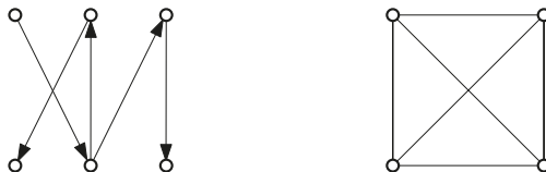
Figure 2.1: Example of a directed, bipartite graph (left) and an undirected, complete graph (right).
