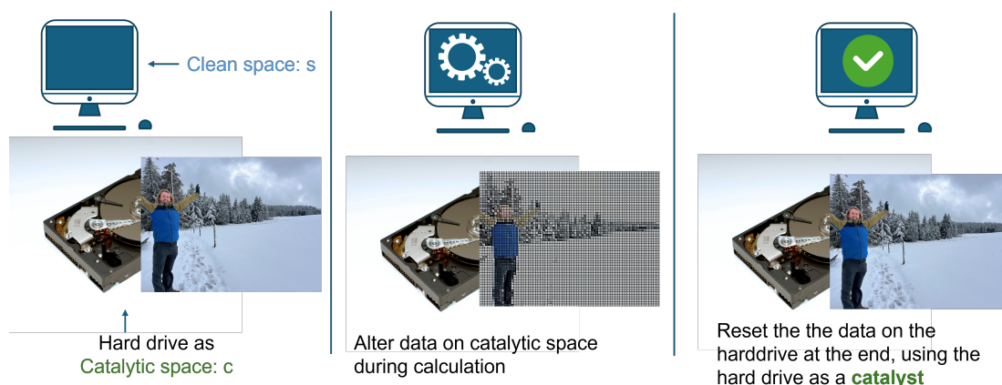
Figure 4.1: An explanatory graphic illustrating catalytic computing. The space-bounded machine (the “clean space”: s ) is represented by the computer, while the catalyst is depicted as a hard drive containing holiday images. During computation, the machine may temporarily alter these images, but by the end, the hard drive is restored exactly to its original state.
