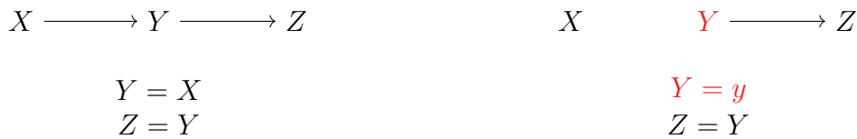
Figure 6.33: A chain (left) and the result of intervening to set Y = y (right).
