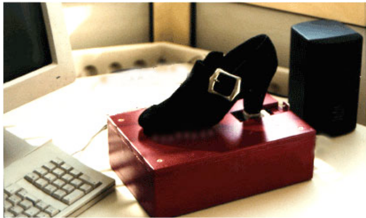
Mechanical shoe used to demonstrate models of beat induction.
