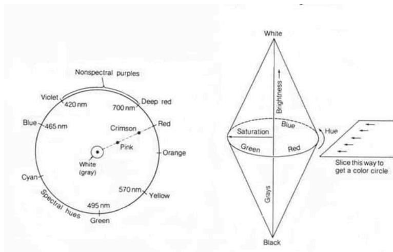
Figure 5.2: The 3D colour spindle.
