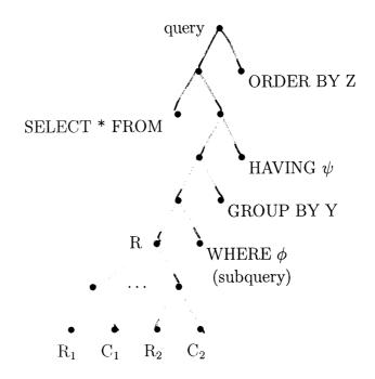
Figure 4: The structure of an SQL query
