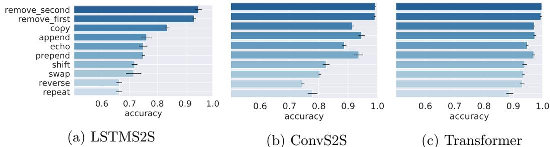
Figure 4.7: Accuracy of the three models per PCFG SET function, as computed by applying the different functions to the same complex input sequences.
