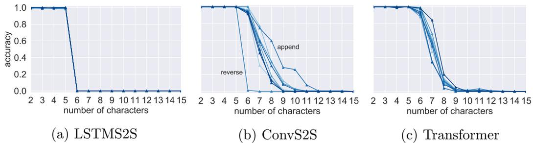
Figure 4.10: Accuracy of the three architectures on different functions with increasingly long character string inputs. The maximum character string length observed during training is 5. While Transformer and ConvS2S can, for most functions, generalise a little beyond this string length, LSTMS2S models cannot.
