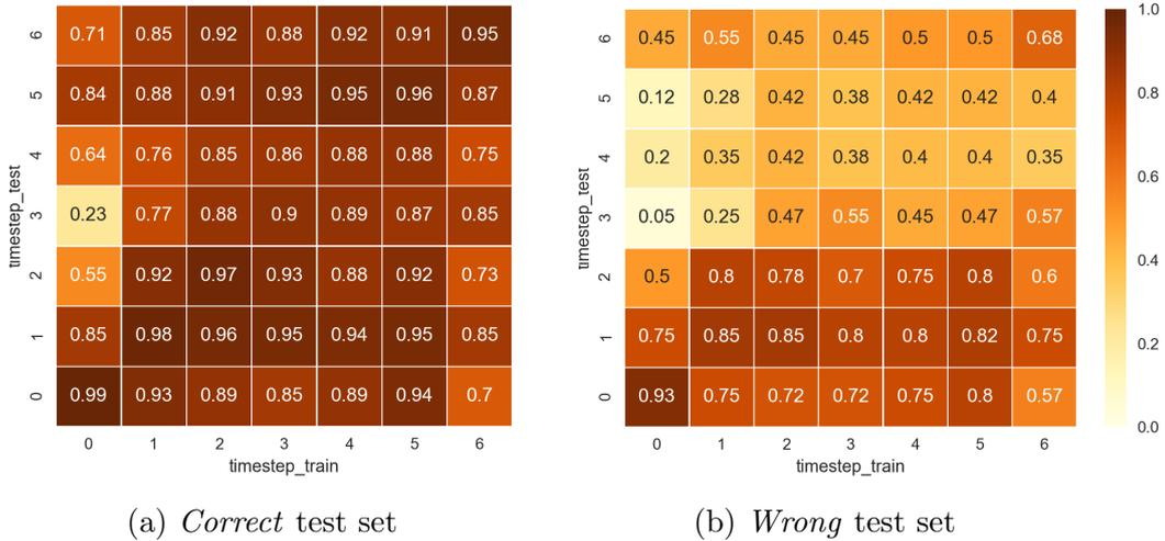
Figure 5.3: The temporal generalisation matrices for diagnostic classifiers trained on memory cell activation at different timesteps, for correct (left) and wrong (right) sentences. Timestep 0 corresponds to the subject of the sentence, the attractor and main verb of the sentence occur at timesteps 3 and 6, respectively. The corpus used for testing is *WD-K\*-L5-M\*-A3*.
