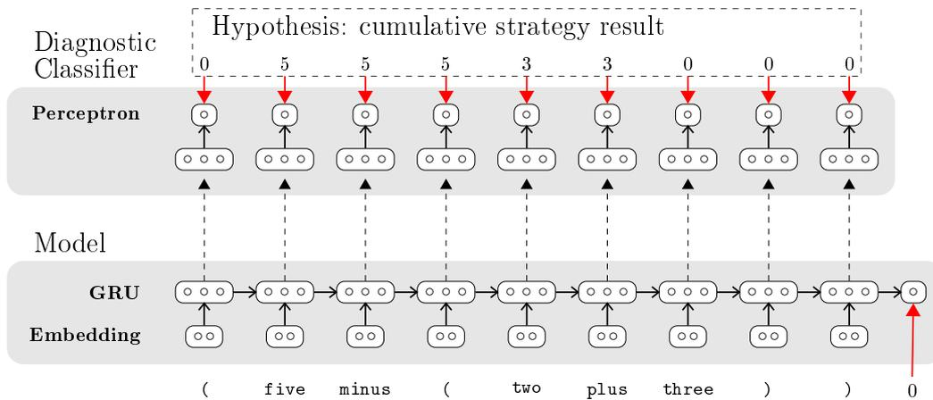
Figure 3.7: Testing a single hypothesis with a diagnostic classifier.
