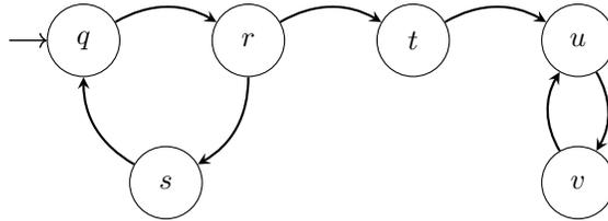
Figure 4.1: Strongly connected components:  $\{q, r, s\}$  and  $\{u, v\}$ .
