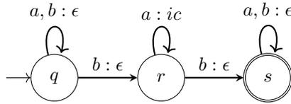
Figure 3.3:  $B$ -automaton recognising  $\text{minblock}_a$ .
